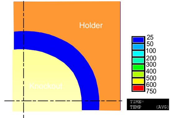
FEM simulation of temperature distribution in local heating
