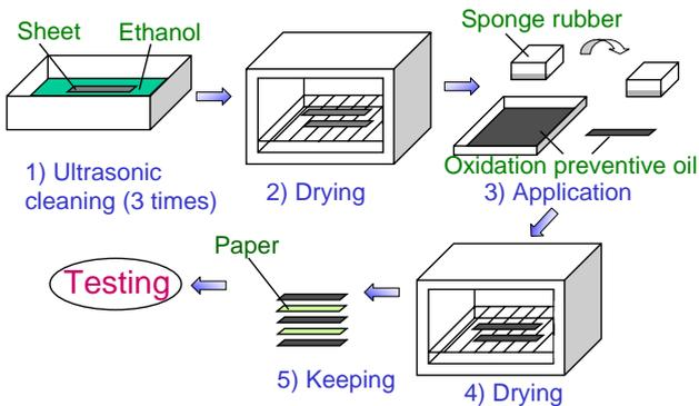
Resistance heating of sheet for evaluation of oxidation preventive oils
