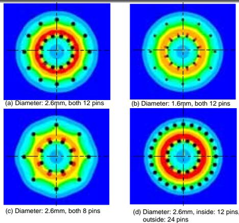
Local heating using contact pins
