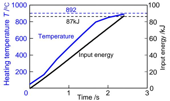
Relationship between measured heating temperature and input energy
