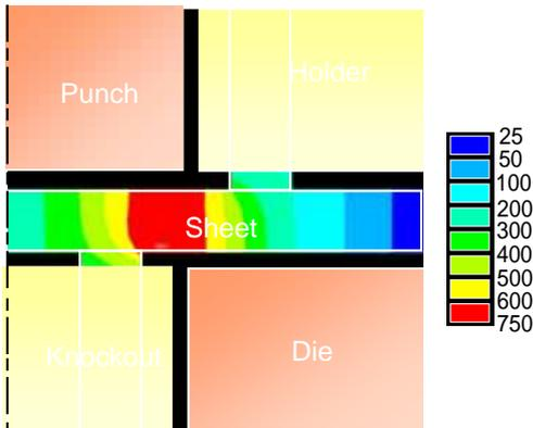
FEM simulation of temperature distribution in local heating
