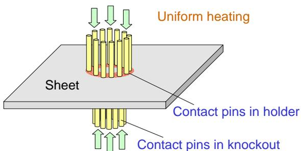
Local heating using contact pins
