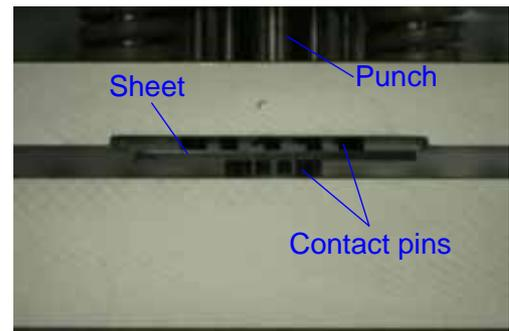
Punched sheet for  $c=10\%$  and  $v=150\text{mm/s}$
