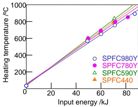
Energy efficiency of resistance heating
