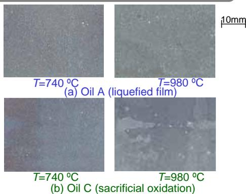
Relationships between scale thickness and heating temperature for different oxidation preventive oils
