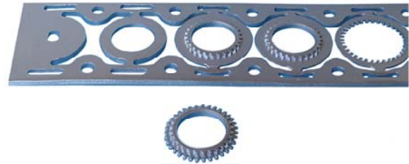
Fig. 14. Forming sequences in progressive dies for double gear [13].
