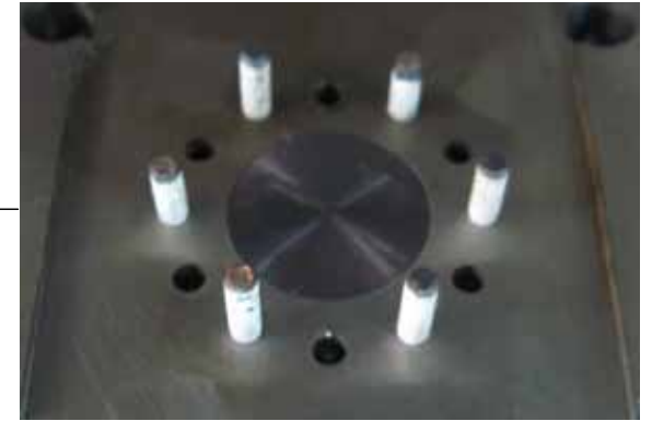
板押え側ピン電極 (Ag-W, Cu-W, Ag+WC, W)
